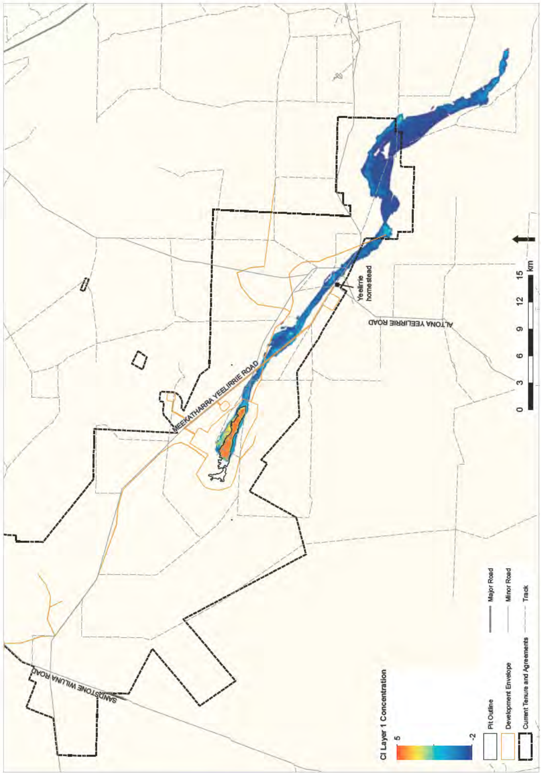
Figure 9-48: Simulated chloride transport plume in model layer 1 at year 15,000
